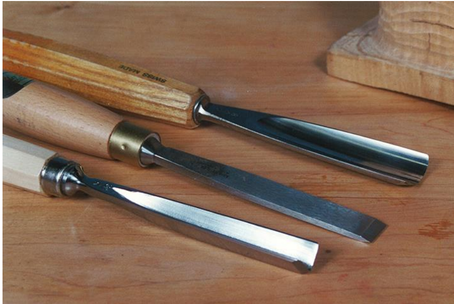
FIGURE 3 TRADITIONAL WOOD CARVING TOOLS – V-TOOL, CHISEL, GOUGE
