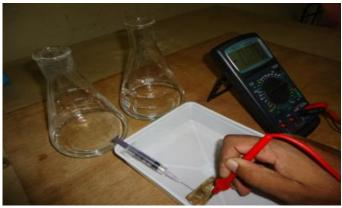
**Figure. 3. (b)** Figure.1, 2 shows the basic biosensor Figure.3(a),(b) shows the voltages for the analyte – Glucose oxidase on collagen biosensor for hypo and hyper glycemic levels.
