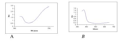
**Fig.3.** Visible absorption spectra of (A) chromogenic reagents (Fe(III) +  $[Fe(CN)_6]^{3-}$ ) and (B) (A) + acidic hydrolysis products of Tetracycline .
