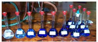
Fig.1. Different concentrations of antibiotics for drawing calibration curve.
