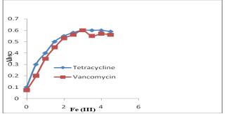
Fig. 7. Ef fect of different concentrations of [Fe(III)]on the absorbance of PB complex produced correspond ing to: Tetracycline and Vacomycin.
