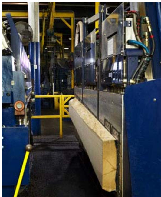
Figure 4: Vacuum Table and Backer Board Merritt PMI (2006)
