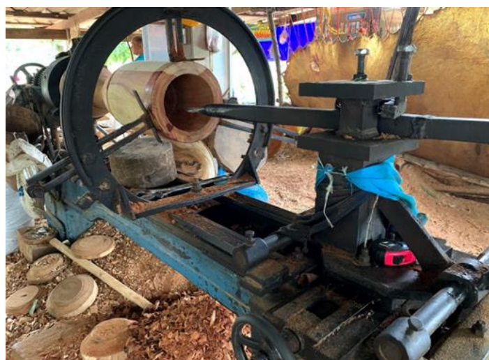
FIGURE 3 CORING ISAN FOLK LONG DRUMS
