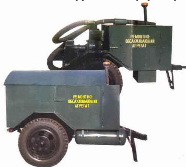
FIGURE 5 TRAILED REPAIRS-MAINTENANCE UNIT PROA-1
